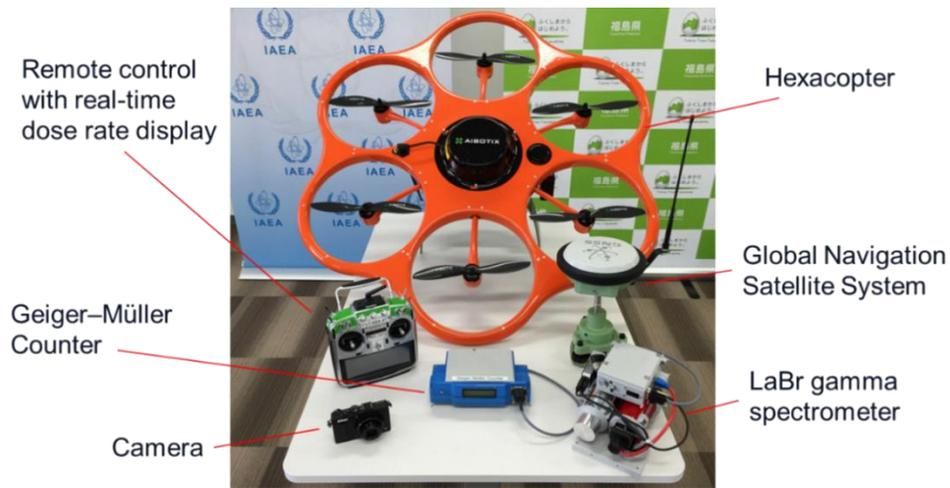
FIG. 5.1: UAV-based system and its instrumentation components delivered to the Prefecture. Image: IAEA.
