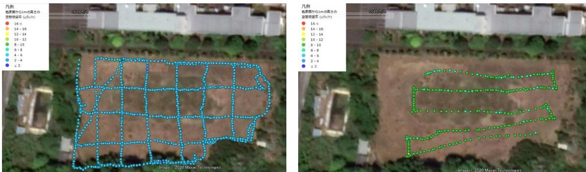
FIG. 5.2: Example of in situ measurements (not corrected raw data) performed in the area accessible both for backpack and UAV techniques: data points obtained with the UAV system (Geiger-Müller counter) flying at 10m altitude (on the left); data points obtained with backpack system (CsI spectrometer) walking throughout the area with the detector located at 1m altitude (on the right). Image: Fukushima Prefecture.
